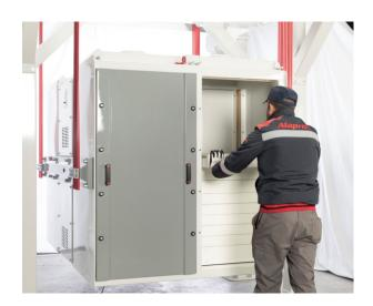
Passages doors are made of fiberglass with a bright and smooth surface, using insulation to prevent condensation, are manufactured using the cast method and have a highly resistant structure.
